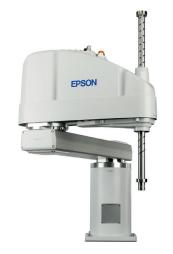
The Epson SCARA G20 is suitable for very high loads with a weight of up to 20kg. An arm length of 1,000 or 850mm ensures that a large working area is covered. Due to the high moment of inertia of the U axis, heavy loads can be moved quickly and reliably – without vibrations of the robot's arm that is often found with many competing models with a similar arm length.
