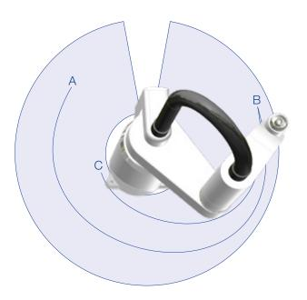
Conventional SCARA robots: Kidney-shaped working range with dead zone
